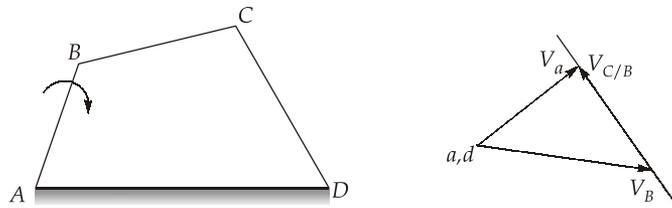
Points *a* and *d* given on fixed link are represented by a single point as shown in velocity diagram.
