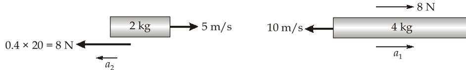
$$\begin{aligned} \therefore a_2 &= -\frac{8}{2} = -4 \text{ m/s}^2 \\ a_1 &= \frac{8}{4} = 2 \text{ m/s}^2 \end{aligned}$$
