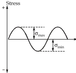
For a completely reversed stress condition,
