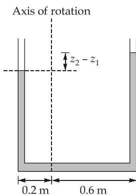
$$(z_2 - z_1) = \frac{\omega^2}{2g} (x_2^2 - x_1^2) \quad \dots(i)$$
