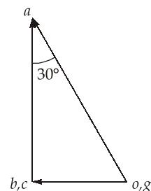
$$V_{ao} = \omega r = \frac{2\pi \times 180}{60} \times 15 = 90\pi \text{ cm/s}$$
