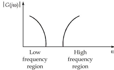
Magnitude v/s  $\omega$  curve of lag-lead compensator.
