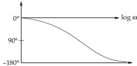
As phase angle curve never crosses  $-180^\circ$  line, therefore phase crossover frequency does not exist i.e.  $\omega_{pc}$  is infinite and gain margin is also infinite.
