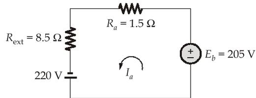
The armature current during plugging,
