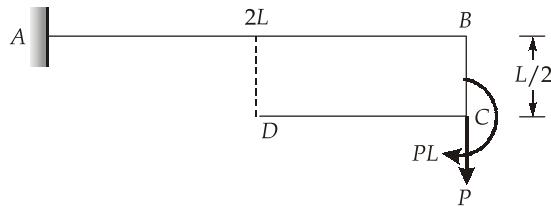
The force can be transmitted at end C as shown.
