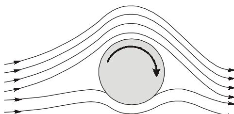
On upper side of cylinder fluid and boundary are moving in same direction so no formation of boundary layer will occur. This is one of the famous method to avoid boundary layer separation.
