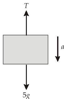
Acceleration for A will be upwards and for B and C will be downwards. Applying Newton's law to the block C.
