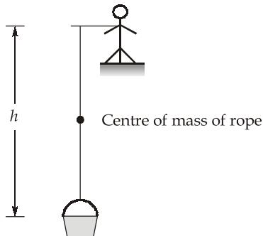
The centre of mass of the rope rises by  $\frac{h}{2}$  and the centre of mass of the bucket rises by  $h$ .
