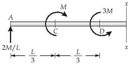
$$\begin{aligned} BM &= \frac{2M}{L}x + M - 3M \\ &= \frac{2M}{L}x - 2M \end{aligned}$$
