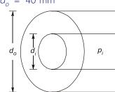
Internal pressure,  $p_i = 100 \text{ MPa}$
