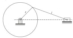
Given: Radius of crank, r = 30 mmLength of connecrting rad, l = 120 mmRevolution per minut, N = 60 rpm
