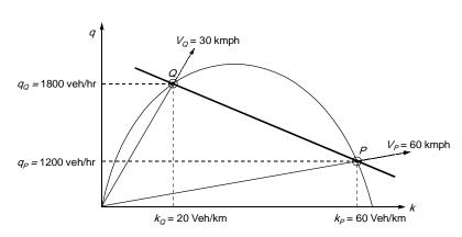
Speed of shock wave (PQ) is, slope of line PQ,
