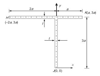
The coordinates of the shear center of this cross-section are:
