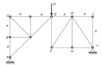
The magnitude (absolute value) of force (in kN) in member EF is \_\_\_\_\_. (round off to the nearest integer)
