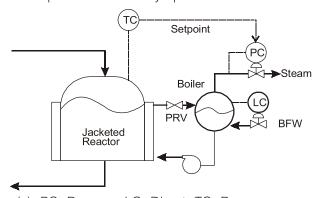
LC: Level Controller PC: Pressure Controller
