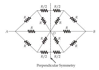
Here, O is equipotential point. Along the perpendicular (dotted line) point O is separated because no current flows at point O.
