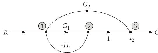
Forward paths :  $P_1 = G_1$  ; $P_2 = G_2$ Loop :  $L_1 = -G_1 H_1$ Loop touches both forward paths so  $\Delta_1 = \Delta_2 = 1$ and  $\Delta = 1 - L_1 = 1 + G_1 H_1$
