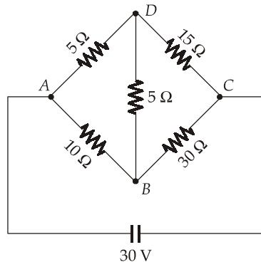
The above circuit is balanced Wheatstone's bridge. Hence current  $I$  through  $5\Omega$  resistor i.e. between  $B$  and  $D$  is 0.
