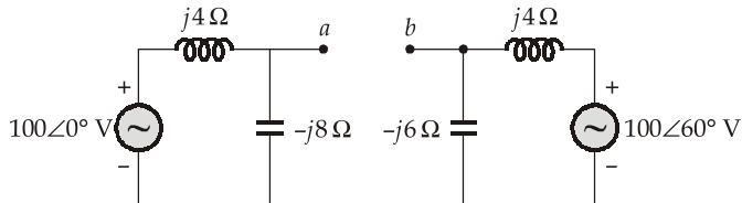
$$V_a = \frac{100\angle 0^\circ}{j4 - j8}(-j8) = 200\angle 0^\circ \text{ V}$$
