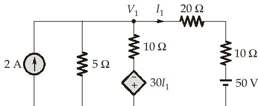
$$I_1 = \frac{V_1 - 50}{20 + 10} = \frac{V_1 - 50}{30}$$
