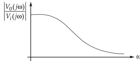
So the circuit is low pass filter.
