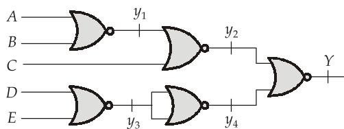
$$y_1 = \overline{A+B}, \quad y_2 = \overline{y_1+C}$$
