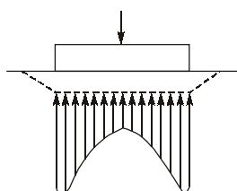
**(iii) Flexible footing on granular soil**
