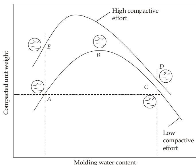
The more orderly, nearly parallel orientation of particles allows the particles (point C and D) to pack more efficiently as compared to the randomly oriented particles on the dry side of optimum.
