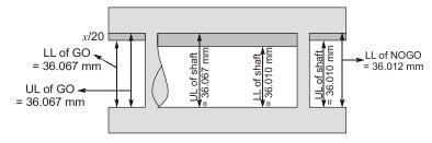
Tolerance of shaft (x) = 36.070 - 36.010= 0.060 mm
