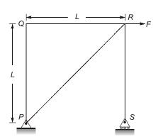
The forces in the members PR and RS, respectively, are \_\_\_\_\_\_.
