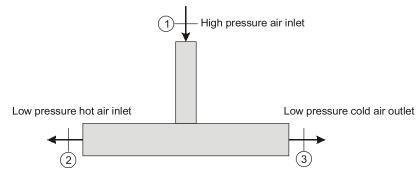
Consider constant specific heat of air is 1005 J/kg.K and gas constant is 287 J/kg.K. There is no work transfer across the boundary of this device. The rate of entropy generation is \_\_\_\_\_\_ kW/K (round off to one decimal place).
