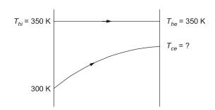
$$NTU = \frac{UA}{(\dot{m}c_p)_{\text{small}}} = \frac{1500 \times 400}{100 \times 4000} = 1.5$$
