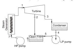
Specific enthalpy of steam at location 2 is 2624 kJ/kg, specific enthalpy of water at location 5 is 226.7 kJ/kg and specific enthalpy of saturated water at location 6 is 708.6 kJ/kg. If the mass flow rate of water entering the open feed water heater (at location 5) is 100 kg/s then the mass flow rate of steam at location 2 will be\_\_\_\_\_kg/s (round off to one decimal place).
