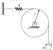
The pulley radius is r and its mass moment of inertia is J. Assume that the mass is vibrating harmonically about its static equilibrium position. The natural frequency of the system is
