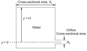
Neglecting any losses, the time taken by water in the tank to reach a level of y = H/4 is \_\_\_\_\_ seconds (round off to one decimal place).
