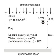
The primary consolidation settlement (in m, round off to two decimal places) of the clay layer resulting from this loading will be \_\_\_\_\_\_.
