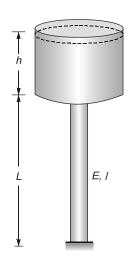
If elastic modulus (*E*) of steel is 200 GPa, ignoring self-weight of the tank, for the supporting steel column to remain unbuckled, the maximum depth (h) of the water permissible (in m, round off to one decimal place) is \_\_\_\_\_\_.
