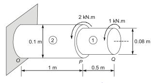
$$\tau_{\text{max}_{OP}} = \frac{16T_{OP}}{\pi d_{OP}^3} = \frac{16 \times 3 \times 10^3}{\pi \times 100^3} = 15.27 \text{ N/mm}^2$$
