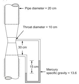
Assume g = 9.8 m/s<sup>2</sup>. When the deflection in the mercury manometer is 15 cm, the flow rate (in lps, round off to two decimal places) considering no loss in the venturimeter is
