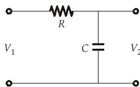
$$\frac{V_2}{V_1} = \frac{1/Cs}{R + 1/Cs} = \frac{1}{1 + RCs}$$
