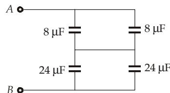
$$C_{\text{eq}} = (8+8)\mu\text{F} \parallel (24+24)\mu\text{F}$$
