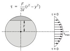
Variation of  $\tau$  versus y is a parabolic curve.
