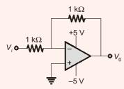
Given circuit is a Schmitt trigger of non-inverting type.
