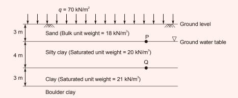
Immediately after preloading, the effective stresses (in kPa) at points P and Q respectively,
