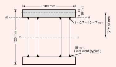
q =Shear stress at the level mn in the weld = 100 MPa =  $\frac{FA\overline{y}}{Ib}$
