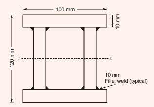
The maximum shear force (in kN, round off to one decimal place) that can be carried by the section, is \_\_\_\_\_.
