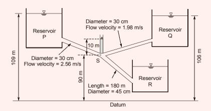
Considering head loss only due to friction (with friction factor of 0.03 for all the pipes), the height of water level in the lowermost reservoir R (in m, round off to one decimal places) with respect to the datum, is \_\_\_\_\_.
