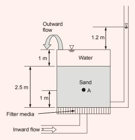
The effective stress (in kPa, round off to two decimal places) at point A, located 1 m above the base of tank, is \_\_\_\_\_.
