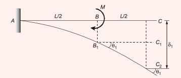
$$\begin{split} \delta_c &= \delta_1 = CC_1 + C_1C_2 \\ &= BB_1 + C_1C_2 \\ &= \frac{M\left(\frac{L}{2}\right)^2}{2EI} + \frac{M\left(\frac{L}{2}\right)}{EI} \left(\frac{L}{2}\right) \end{split}$$
