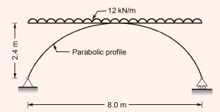
Neglecting self-weight, the maximum bending moment generated in the structure (in kNm, round off to the nearest integer), is \_\_\_\_\_\_.
