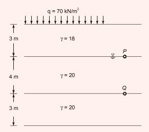
Surcharge (q = 70 kN/m<sup>2</sup>) is applied instantaneously hence excess pore pressure  $(u_i = 70 \text{ kPa})$  is developed at point P and Q [GWT level is at level P]
