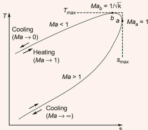
Entropy increases with heat gain, and thus we proceed to the right on the Rayleigh line as heat is transferred to the liquid. The Mach number is  $Ma = 1$  at point a, which is the point of maximum entropy.
