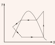
Liquid sub-cooler always increases the refrigeration effect (RE) of cycle.
