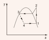
$h_1 = 232 \text{ kJ/kg}, h_2 = 283 \text{ kJ/kg}, h_3 = 116 \text{ kJ/kg}.$  $COP = \frac{h_1 - h_4}{h_2 - h_1} = 2.27$
