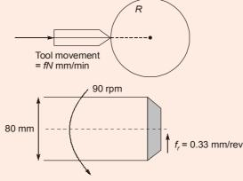
Machining time  $(t_m)$  in facing operation =  $\frac{R}{fN} = \frac{D/2}{f_r N} = \frac{40 \text{ mm}}{0.3 \frac{\text{mm}}{\text{rev}} \times 90 \frac{\text{rev}}{\text{min}}} = 1.48 \text{ min}$
