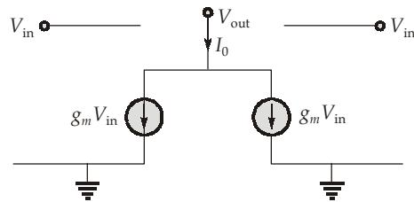
$$g_{m(\text{net})} = \frac{I_0}{V_{in}} = \frac{g_m V_{in} + g_m V_{in}}{V_{in}} = 2 g_m$$
