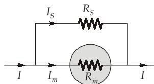
Shunt resistance,  $R_{sh} = 2 \times 10^{-3} \Omega$
