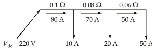
$$\begin{aligned}V_{\min} &= V_{dc} - I_1 R_1 - I_2 R_2 - I_3 R_3 \\&= 220 - (80 \times 0.1) - (70 \times 0.08) - (50 \times 0.06) \\&= 203.4 \text{ V}\end{aligned}$$
