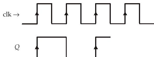
and  $Q$  is input to MOD-3 counter then after 3 clock pulses of input clk there are 2 +ve edge of clock input  $Q$  so output of counter goes to  $2 = (10)_2$
