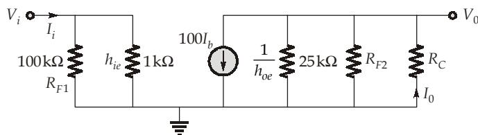
$$R_i = (R_{F1} \parallel h_{ie}) = \frac{100 \times 10^3 \times 1 \times 10^3}{(100 + 1) \times 10^3} = 0.99 \text{ k}\Omega$$
