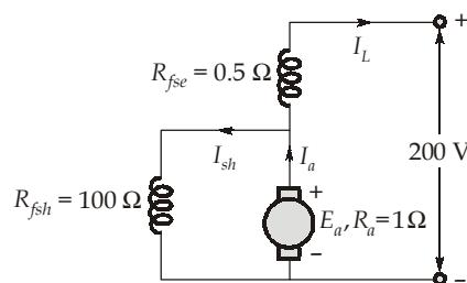
$$\text{Load current} = \frac{\text{Load power}}{\text{Terminal voltage}} = \frac{4000}{200} = 20 \text{ A}$$
