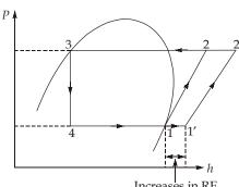
As pressure ratio remains same the volumetric efficiency of compressor will remain same. Due to superheating, specific volume of refrigerant will increase hence the compressor work will increases.
