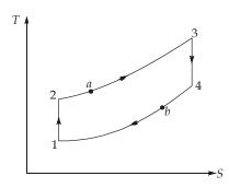
Effectiveness of regenerator,  $\dot{\varepsilon} = \left(\frac{T_a - T_2}{T_4 - T_2}\right)$
