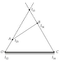
About  $I_{13}$ , link 3 is in pure rotation as link 1 is fixed. Clearly velocity of A will be greater as  $I_{13}I_{23} > I_{13}I_{34}$
