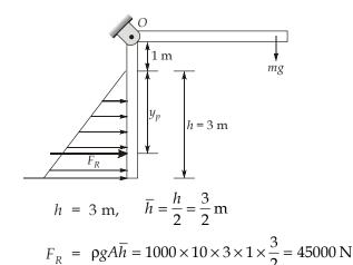
Centre of pressure,  $y_p$  = Centroid of triangular prism =  $\frac{2}{3}h = \frac{2}{3} \times 3 = 2$  m  $mg \times 6 = F_R (y_p + 1)$
