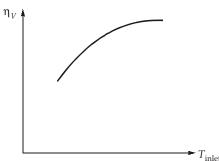
Mass of air  $m_a$  is proportional to  $\rho_i \times \eta_v$ . When inlet temperature increases,  $\eta_v$  does not increases enough to compensate for the reduction in  $\rho_i$  and hence the product  $\rho_i \times \eta_v$  has a lower value.
