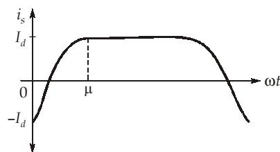
$$\int_0^{\mu} \sqrt{2V_s} \sin \omega t \, d\omega t = \int_{-I_d}^{I_d} \omega L_s \, di_s$$
