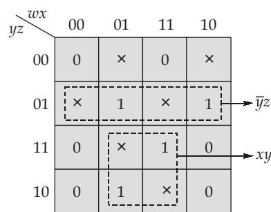
Minimal SOP of the given K-map is  $xy + \bar{y}z$
