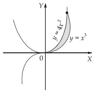
$$\begin{aligned} A &= \int_{x=0}^{4} (4x^2 - x^3) dx \\ &= \left. \frac{4x^3}{3} - \frac{x^4}{4} \right|_{x=0}^4 = \frac{256}{3} - \frac{256}{4} \\ &= \frac{256}{12} = \frac{64}{3} \end{aligned}$$
