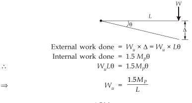
So, collapse load for beam is  $\frac{1.5M_P}{L}$
