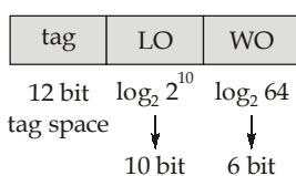
$$\begin{aligned}\text{Tag directory size} &= \text{No. of lines in CM} \times \text{tag space} \\ &= 2^{10} \times 12 \text{ bit} = 1024 \times 12 \text{ bit}\end{aligned}$$
