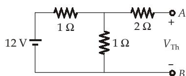
$$V_{Th} = 12 \times \frac{1}{1+1} = 6 \text{ V}$$
