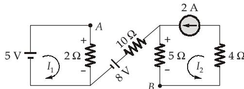
$$\text{Potential difference, } V_{AB} = V_A - V_B$$
