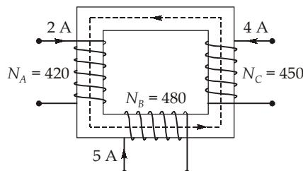
flux by coil-B and coil-C are in same direction, in opposition of coil-A.
