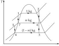
For the regenerative steam cycle considered, with unit mass of steam leaving boiler and 'm' kg of steam bled out for feed water heating:
