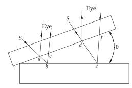
The two reflected components of the light ray are collected and recombined by the eye, having travelled two different paths whose length differs by an amount 'abc'. if 'abc' =  $\frac{\lambda}{2}$ , where  $\lambda$  is the wavelength of the monochromatic light source, then the condition for complete interference has been satisfied. The eye is now able to see a distinct patches of darkness termed a as fringe.
