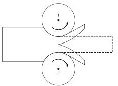
Alligatoring: Rolled object split open in the middle due to friction and high forces at roll surface.
