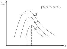
The radiation emitted by the sun, which is considered to be a blackbody at 5780K, reaches its peak in visible region of spectrum. Therefore, the sun is in tune with our eyes. On the other hand, surfaces at  $T \le 800$ K emit almost entirely in infrared region and thus are not visible to eye unless they reflect light coming from other sources.
