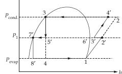
As two compressors (1 - 2' and 3' - 4') are used and two 2 throttling devices (3 - 5' and 7' - 8') are used the cost of equipment will increases. For same size of evaporator, the mass flow rate through evaporator will be same so refrigeration effect has been increased from  $(h_1 - h_4)$  to  $(h_1 - h_{8'})$
