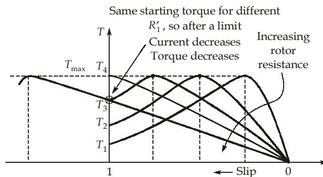
As  $R$  increases, starting torque increases upto maximum torque ( $T_4 = T_{\text{max}} > T_3 > T_2 > T_1$ ) but rotor consumes more power so copper loss increases and efficiency decreases.
