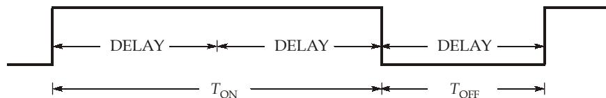
$$\text{Duty cycle} = \frac{T_{ON}}{T_{ON} + T_{OFF}} \times 100 = \frac{2}{3} \times 100 = 66.66\% \simeq 66\%$$
