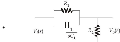
it act as lead compensator (high-pass filter), which improves transient response but steady state performance is not much effected.
