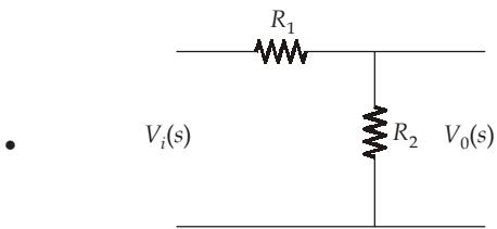
which is a simple resistive network, and it attenuates the gain i.e.,  $\frac{V_0(s)}{V_i(s)} = \frac{R_2}{R_1 + R_2}$ .
