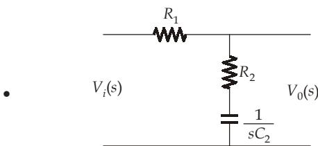
it acts as a lag compensator (low-pass filter), which reduces the bandwidth.
