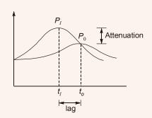
The outflow from the reservoir is uncontrolled therefore peak of outflow hydrograph will occur at the junction of inflow and outflow hydrograph.
