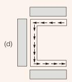
Ans. (c) Shear flow distribution for channel.
