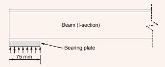
As per IS: 800-2007, the web bearing strength (in kN, round off to 2 decimal places)
