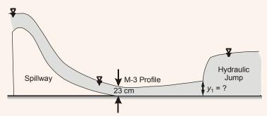
The flow enters as an M-3 profile in the long wide rectangular channel with bed slope
