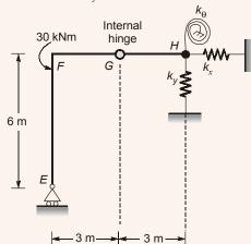
For the externally applied moment of 30 kNm at node F, the rotation (in degrees, round off to 3 decimals) observed in the rotational spring at node H is\_\_\_
