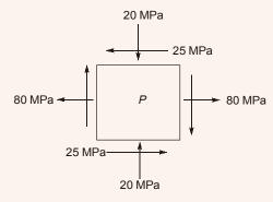
By how much angle  $(\theta)$  in degrees the stress element should be rotated in order to get the planes of maximum shear stress?
