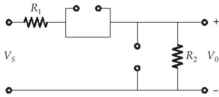
$$\frac{V_0}{V_S} = \frac{R_2}{R_1 + R_2}$$
