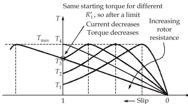
As  $R$  increases, starting torque increases upto maximum torque ( $T_4 = T_{\max} > T_3 > T_2 > T_1$ ) but rotor consumes more power so copper loss increases and efficiency decreases.
