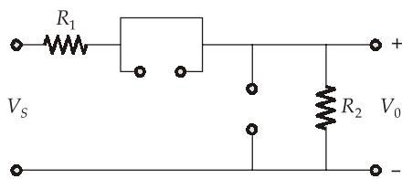
$$\frac{V_0}{V_S} = \frac{R_2}{R_1 + R_2}$$
