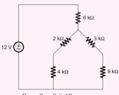
$R_{\rm eq} = 6 + 6 \parallel 12$   $R_{\rm eq} = 6 + 4 = 10 \text{ k}\Omega$
