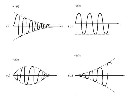
**Q.164** A system having transfer function,  $\frac{C(s)}{R(s)} = \frac{1}{s^2 + 1.5s + 4}$  is subjected to a step input having
