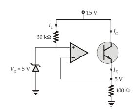
$$V_0 = 5 \text{ V}$$
