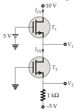
The two N-MOS transistor are identical with threshold voltage  $V_T = 1$  V and  $\frac{\mu_n C_{ox} W}{L} = 2 \text{ mA}/\text{V}^2$ . Assuming the value of  $\lambda = 0$ , the value of drain to source voltage for transistor  $T_2(V_{DS2})$  is equal to \_\_\_\_\_ V.
