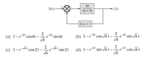
Q.157 The step response of a system is shown below, the forward path gain is \_\_\_\_\_.
