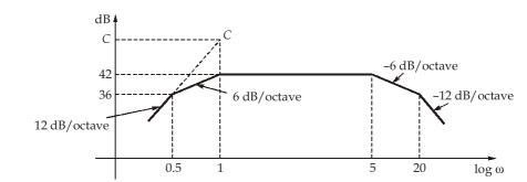
Initial slope of line is 12 dB/octave = 40 dB/decode Finding *k*: at  $\omega = 0.5$  rad/s, M = 36 dB
