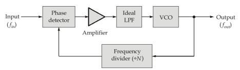
If the reference input frequency  $(f_{in})$  to the above synthesizer is 0.48 MHz and the frequency divider in the feedback path has N = 50, then the steady state output frequency  $(f_{out})$  will be MHz.
