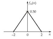
The probability of transmitting  $X = +\alpha$  is "P" and "\alpha" is a positive real value. To get zero probability of error in decision making, the minimum value of " $\alpha$ " should be
