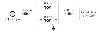
The generator is delivering 1.0 pu power at the instant preceding the fault. The value of critical clearing angle for clearing the fault with simultaneous opening of the breakers 1 and 2 is
