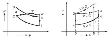
All the cycles start from the same initial state point 1 and the air is compressed from state 1 to state 2 as the compression ratio is same. From the T-s diagram, it can be seen that for the same heat input, heat rejection in diesel cycle (514'6') is maximum and more than that in otto cycle (5146). Consequently, the otto cycle has the highest work output and efficiency.
