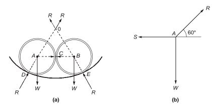
S = Reaction between the two spheres at C.
