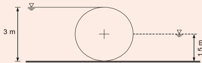
Net vertical force due to water on gate
