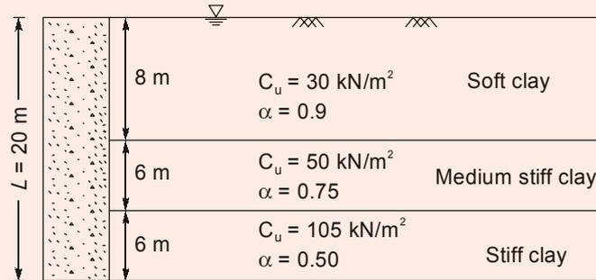
Dia. of pile,  $D = 450 \text{ mm}$
