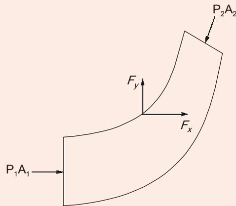
$F_x$  and  $F_y$  = Force exerted by bend on water in  $x$  and  $y$  direction respectively.
