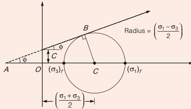
$$\text{In } \triangle ABC, \quad \sin \phi = \frac{BC}{AC} = \frac{BC}{AO + OC} = \frac{\left(\frac{\sigma_1 - \sigma_3}{2}\right)}{c \cot \phi + \left(\frac{\sigma_1 + \sigma_3}{2}\right)} \quad \left(\because \tan \phi = \frac{C}{AO}\right)$$
