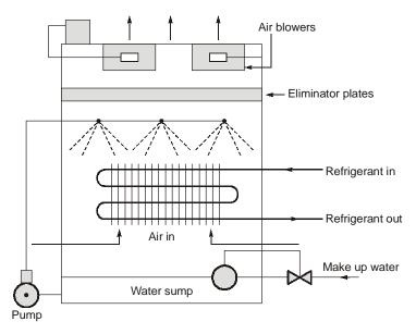
Consider and evaporative condenser as shown above. Water is pumped from the sump and sprayed on tubes carrying refrigerant. Water droplets on tube get evaporated by extracting latent heat of vaporization from refrigerant. Water is continuously recirculated and make up water is added as required.
