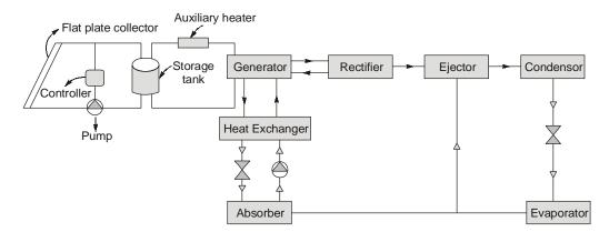
As shown in above diagram, solar heating system supplies heat to the generator. Normally  $NH_3-H_2O$  combination is used as refrigerant and absorber in VAR system.
