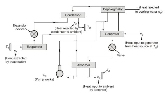
As compared to a vapour compression system differences are:
