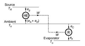
Work output of heat engine is used to power the refrigerator.
