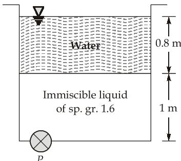
$$\begin{aligned}\text{Total pressure at } P &= \gamma_w \times 0.8 + 1.6 \gamma_w \times 1 \\ &= 2.4 \gamma_w = (2.4 \text{ m of water}) \\ &= 2.4 \times 10000 \\ &= 24 \text{ kPa}\end{aligned}$$
