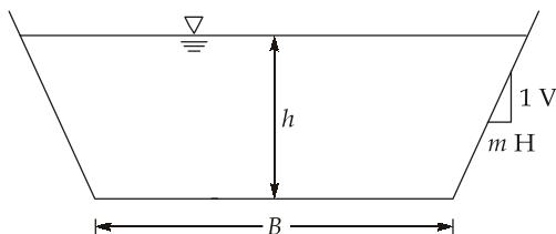
For most efficient trapezoidal section
