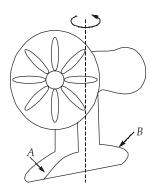
Due to gyroscopic couple, the fan may topple so Monu needs to press at A or B to balance the couple. If fan is rotating in anticlockwise direction when viewed from top, then where do Monu needs to press to balance gyroscopic couple?
