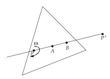
Velocity of point *B* with respect to point '*A*' =  $\omega(PB - PA)$
