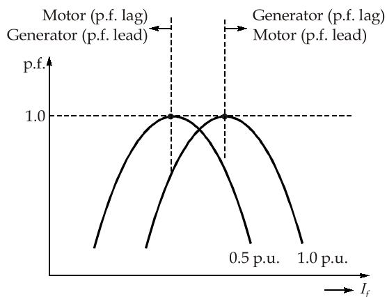
From the diagram above shown if  $I_f$  increases than power factor decreases when generator operates on lagging power factor.
