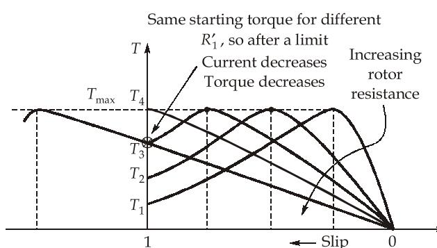
As  $R$  increases, starting torque increases upto maximum torque ( $T_4 = T_{\max} > T_3 > T_2 > T_1$ ) but rotor consumes more power so copper loss increases and efficiency decreases.
