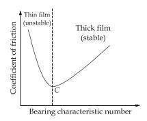
A slight drop in speed (N) or a slight increase in load (P) will reduce the value of bearing characteristic number, resulting in boundary lubrication.
