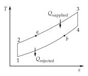
Regeneration cycle is shown in figure. In this cycle heat addition starts at point *a* instead of point 2 from combustion chamber so heat supplied decreases and similarly heat rejection to the surrounding started at point b instead of point 4 so heat rejection also decreases. In the cycle mean temperature of heat addition increases and mean temperature of heat rejection decreases so efficiency of cycle increases.
