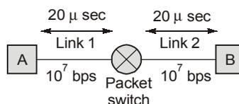
Extra delay at switch =  $35 \mu\text{sec}$  for each packet.
