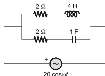
$$\therefore \omega_0 \text{ (resonant frequency)} = \frac{1}{\sqrt{LC}} = \frac{1}{\sqrt{4 \times 1}} = 0.5 \text{ rad/sec.}$$
