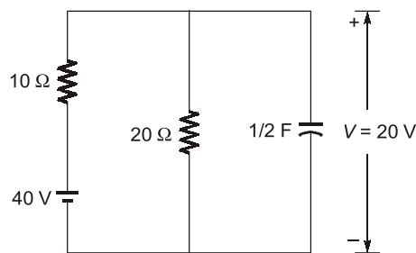
Suppose at time  $t = 0$ , the voltage 'V' = 20 V
