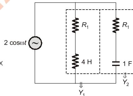
$$\frac{1}{\omega C} \times (R^2 + \omega^2 L^2) = \omega L \left( R^2 + \frac{1}{\omega^2 C^2} \right)$$
