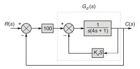
Converting the blocked portion into simplified form as
