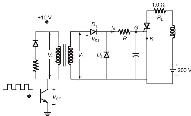
When the pulses are applied to the base of the transistor. Transistor operates in ON state. So, the forward voltage drop in transistor  $V_{CE} = 1 \text{ V}$ .
