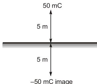
The induced surface charge density is the normal flux density at the point
