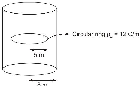
$$\text{Total charge enclosed} = \rho_L \times 2\pi R = 12 \times 2\pi \times 5 = 120\pi \text{ C}$$
